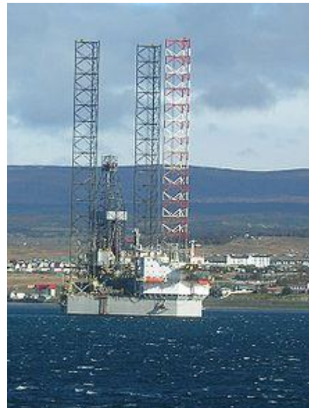
FIGURE F.E1.102.1 – SELF-ELEVATING OR “JACK-UP” UNIT
