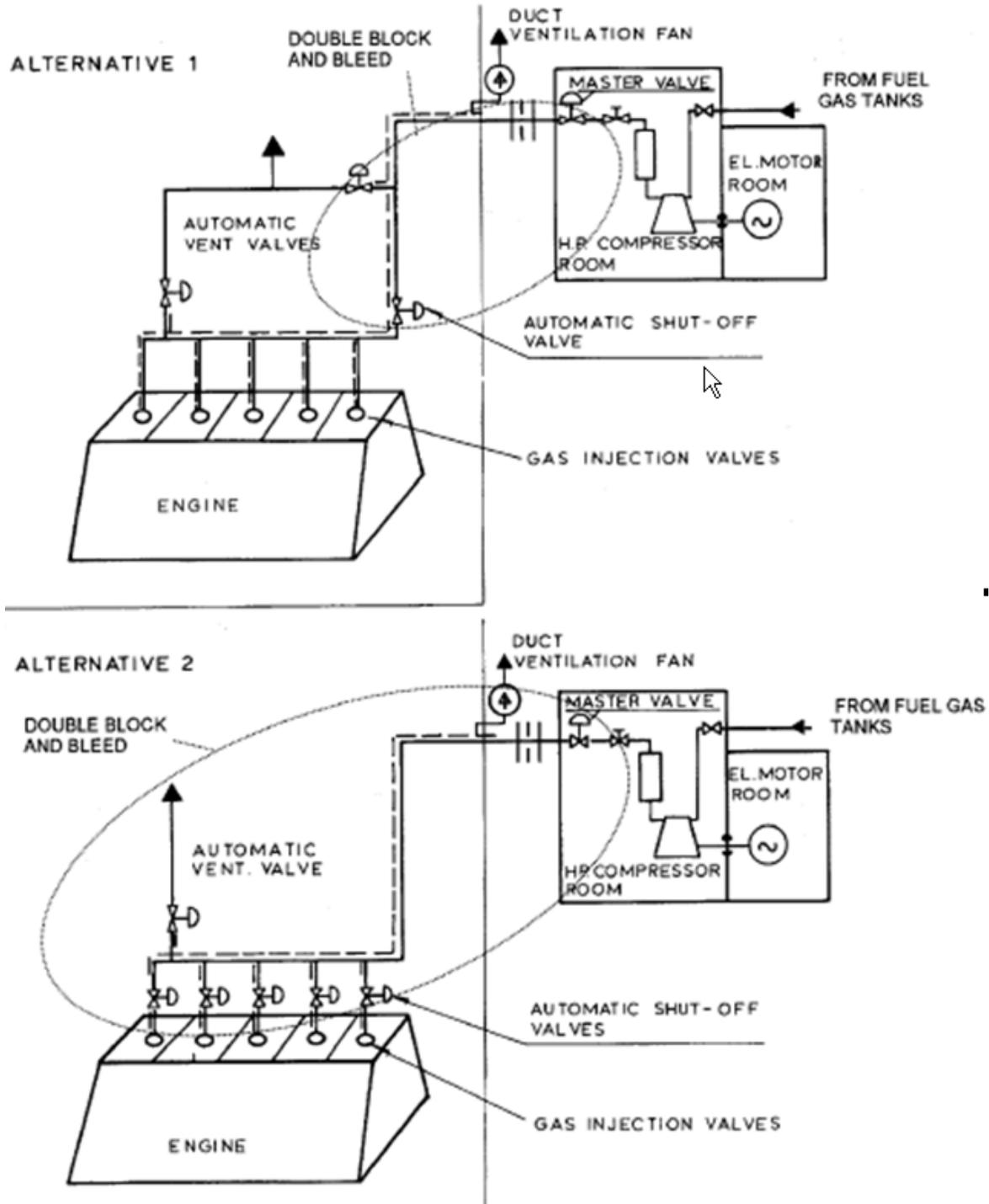
**FIGURE F.F1.603.1 - ALTERNATIVE SUPPLY VALVE ARRANGEMENTS FOR HIGH-PRESSURE INSTALLATIONS (MULTI-ENGINE INSTALLATION)**
